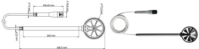
Measuring rangesFrom -5 to 35 m/s<br/>From -20 to +80 °C<br/>From 0 to 99999 m³/hAccuracy\*Air velocity: from 0.4 to 3 m/s:  $\pm 3\%$  of the reading  $\pm 0.1$  m/s<br/>from 3.1 to 35 m/s:  $\pm 1\%$  of the reading  $\pm 0.3$  m/sTemperature Pt100:  $\pm 0.4\%$  reading  $\pm 0.3$  °C<br/>Flow:  $\pm 3\%$  reading or  $\pm 0.03*$  sheath surface (cm²)Resolution0.1 m/s / 0.1 °C / 0.1 m³/h
