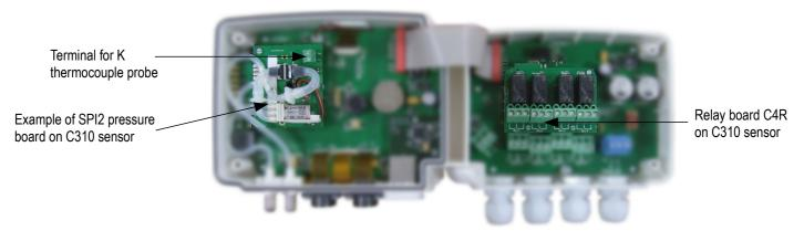
Interchangeable atmospheric pressure board for C310 and CA310 sensors, range 800-1100 hPa. Supplied with pressure fitting and silicone tube.
