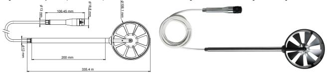
Measuring rangesFrom -5 to 35 m/s<br/>From -20 to +80 °C<br/>From 0 to 99999 m³/hAccuracy\*Air velocity: from 0.3 to 3 m/s:  $\pm 3\%$  of the reading  $\pm 0.1$ m/s<br/>from 3.1 to 35 m/s:  $\pm 1\%$  of the reading  $\pm 0.3$  m/sTemperature Pt100:  $\pm 0.4\%$  reading  $\pm 0.3$ C<br/>Flow:  $\pm 3\%$  reading or  $\pm 0.03^*$  sheath surface (cm²)ResolutionFrom -5 to -3 m/s: 0.1 m/s; from -3 to 3 m/s: 0.01 m/s; from 3 to 35 m/s: 0.1 m/s0.1 °C<br/>0.1 m³/h
